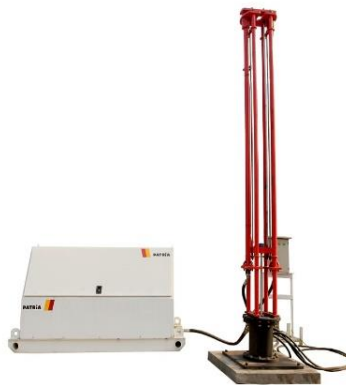
Gambar 1 Hydraulic Pumping Unit
